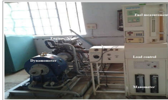
Fig 3.2 Engine connected with dash board
